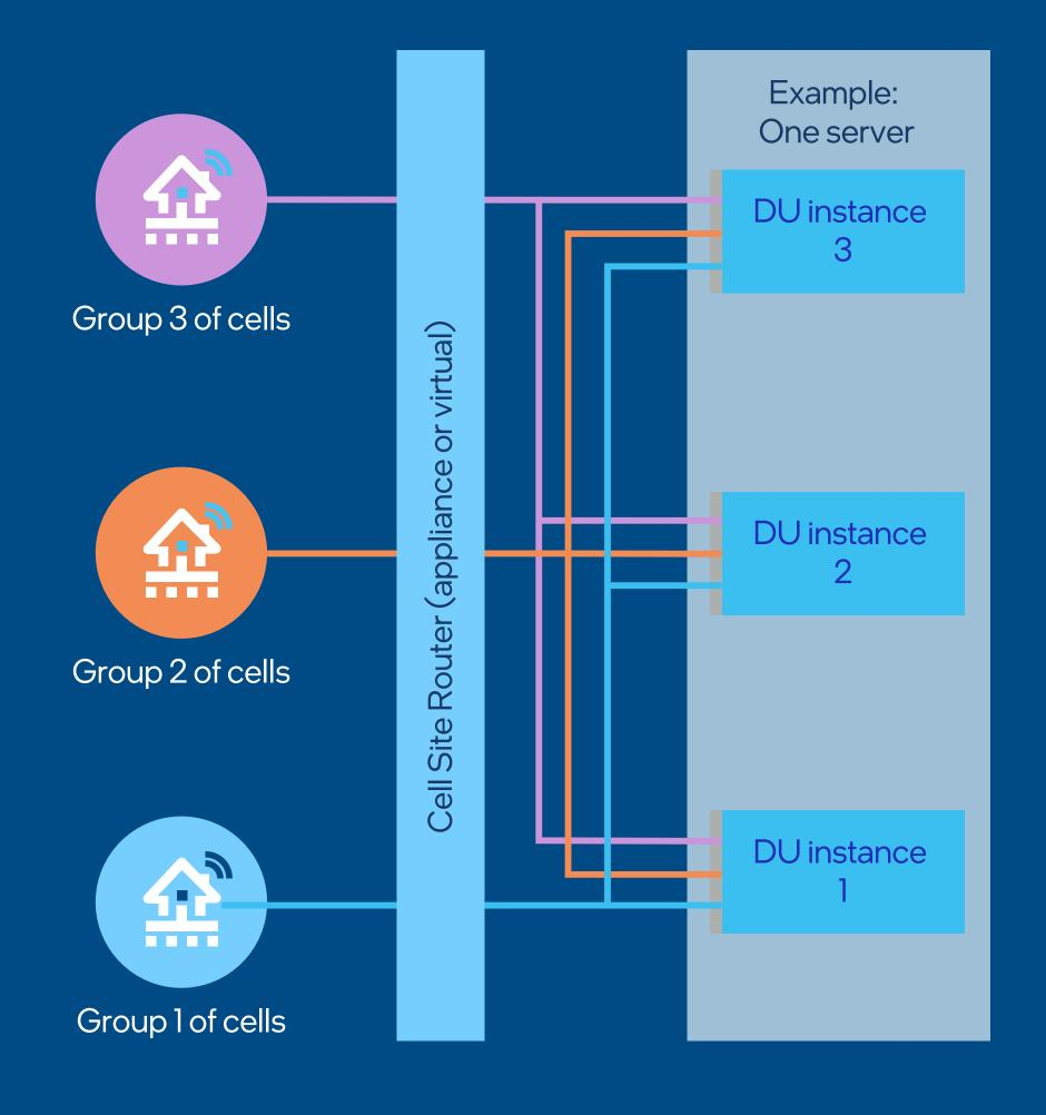
**Figure 1:** Pooling at a site with a single server
