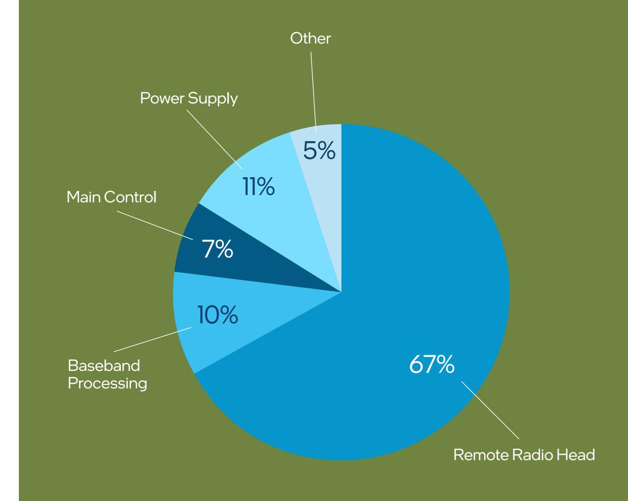
**Figure 2:** Power consumption in a base station without air conditioning<sup>7</sup>
